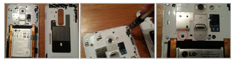
• Use a Phillips #00 screwdriver remove all visible screws.
