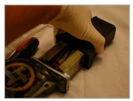
Pull the black plastic electric motor cover away from the gear housing. It does not attach, it's held in place by friction, so a steady pull should move it.
