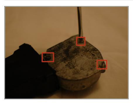
Remove the three flat-head screws on the rear cover of the gear housing.
