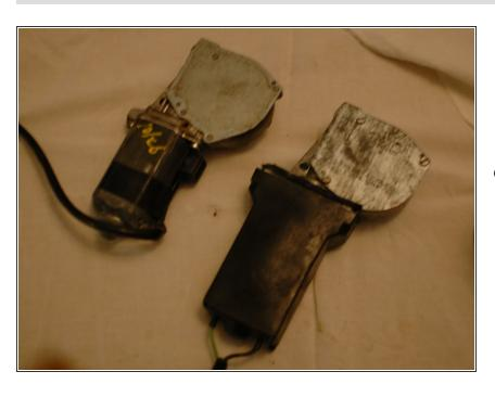
• Before starting this guide, confirm that you are reviewing the guide for the correct motor type for your situation. This guide covers the "Screw Open" style of motor, as seen on the right. If you have a "Drill Open" style of motor as seen on the left click here to review this guide instead.
