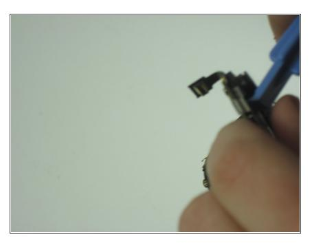
Using the opening tool, detach the camera from the motherboard. To reassemble your device, follow these instructions in reverse order.
