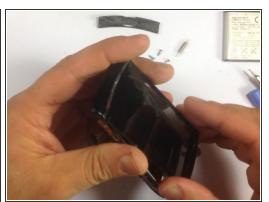
Remove the Touch Screen! To be more easy, heat it with hot air before doing so!
