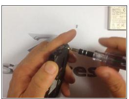
First remove battery, sim card and memory card. You must remove seven screws.
