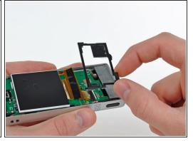
To access the display data cable, use a plastic opening tool to pry the metal and plastic display brackets off the logic board.
