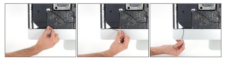
• Gently de-route the power button cable from its groove in the left speaker.
