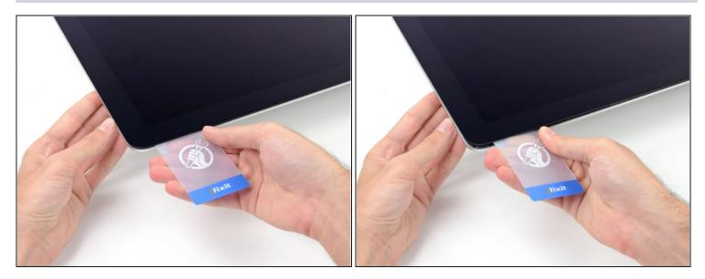
• Gently twist the plastic card to open the space between the display and frame, and cut any remaining adhesive near the corner.
