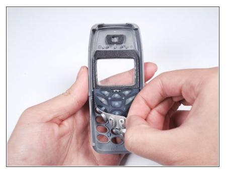
Gently peel up the edge of plastic keypad from the inside of the faceplate to remove.
