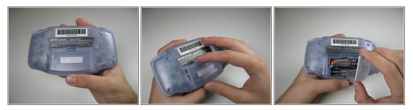
• Take the battery cover off by releasing the locking tab and hinging the cover away. Remove the batteries inside the cover
