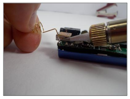
(i) There may be some solder in the way of the spring contacts' metal contacts. If this occurs simply melt the solder to create room for the contacts.
