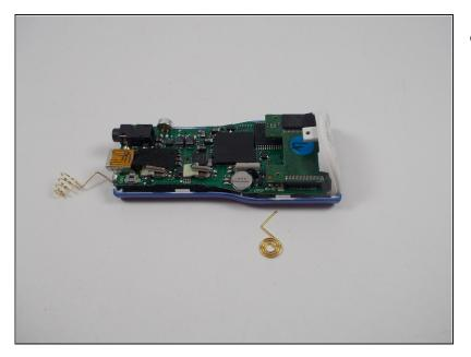
• With solder melted, remove battery spring contacts from the motherboard.
