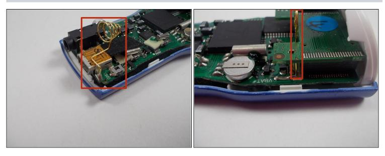
• Locate both battery spring contacts, if necessary, on the motherboard.
