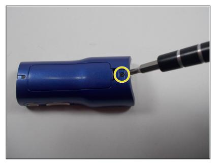
• Locate and remove the screw next to the battery compartment lid.
