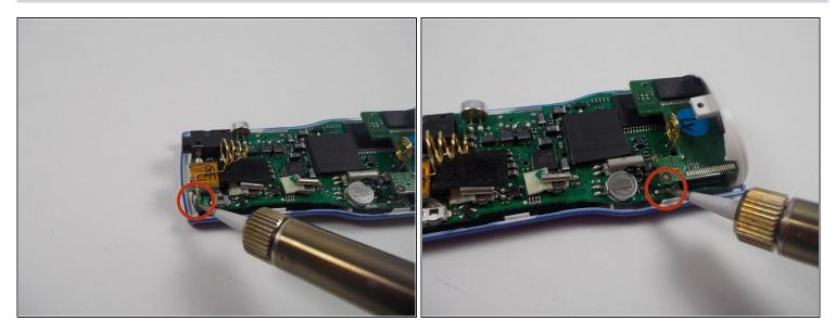
• Apply heated soldering iron to points where the contacts are soldered to the motherboard.
