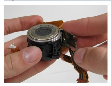
• Lift off the panel, exposing the zoom lens gear drive.
