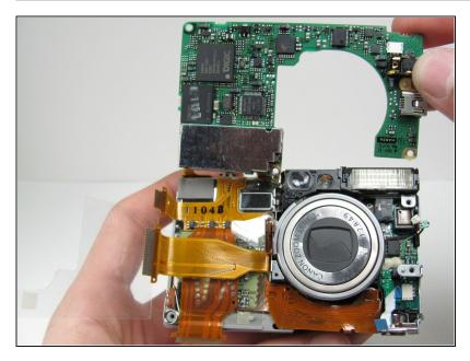
• Free the logic board from the rest of the camera.
