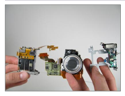
• The remaining pieces from left to right are: the battery casing, zoom lens and flash assembly.
