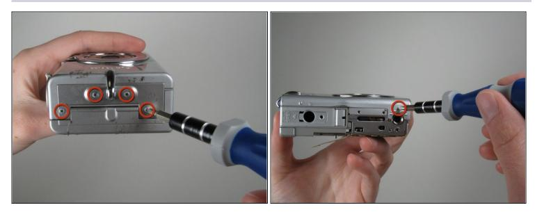
• Unscrew the four Phillips screws from the side of the casing and one screw from the bottom using a #0 Phillips screwdriver.
