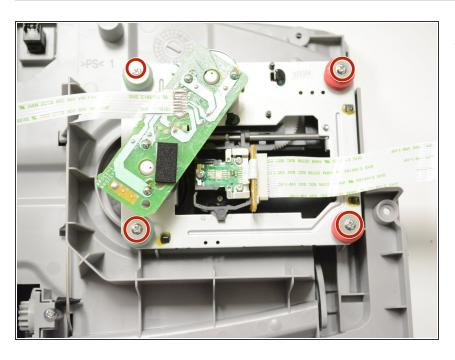
Screw in the new optical pick up unit.
