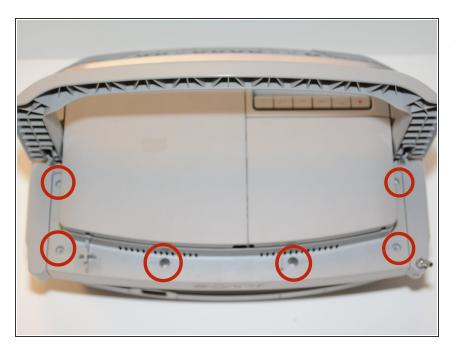
Unscrew the screws on the top of the radio.
