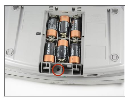
Flip the radio upside down and remove the battery cover. Unscrew the one screw below the batteries.
