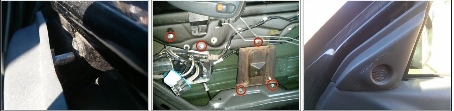
**⚠** Before removing panel, remove small tweeter speaker from top of door panel.. Clipped in just pull the top. Pic 1
