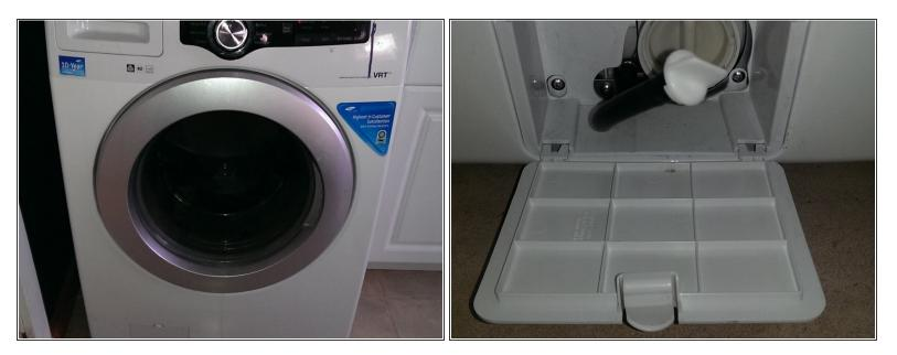
• Remove filter from the lower left corner on the front of the washer
