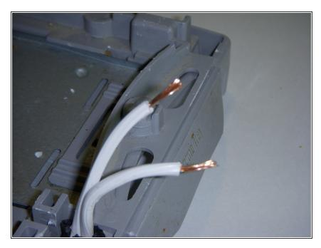
Strip about an inch of the wire insulation (casing) off the ends of both the new power supply cable, and the old power supply cable that is still attached to the toaster.
