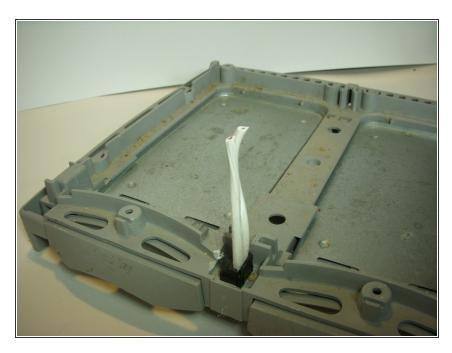
Using wire cutters, cut the power supply cable close to the base of the toaster, leave about 2 inches of wire.
