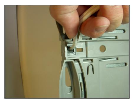
Pull the power supply cord through the bottom plate of the toaster.
