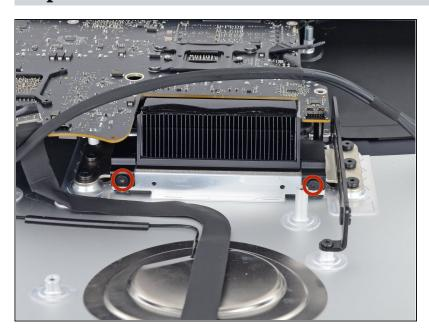
Remove two 5.7 mm T10 screws from the top of the heat sink exhaust duct.
