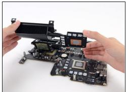
Lift the heat sink up from the logic board.
