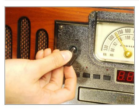
Applying some force, insert the replacement knob onto the peg.
