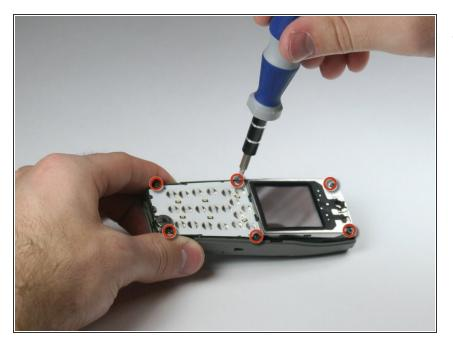
Remove six Torx 6 screws with the screwdriver.
