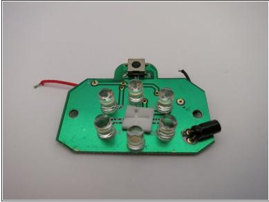
Separate the circuit board from the battery holder by desoldering the black and red wires from the battery holder.
