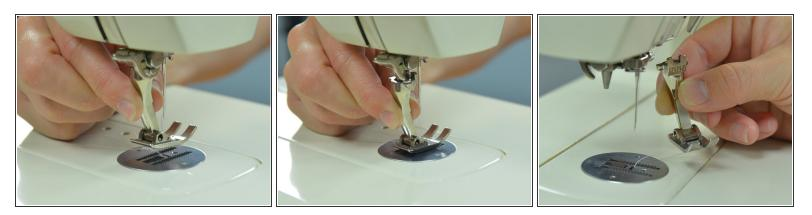
• Pull the presser foot down and slide it off the peg on the machine.
