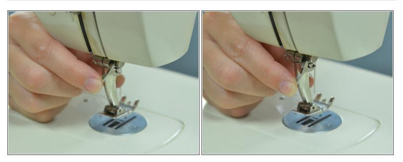
• Slide the presser foot lever down to lock the new foot in place.
