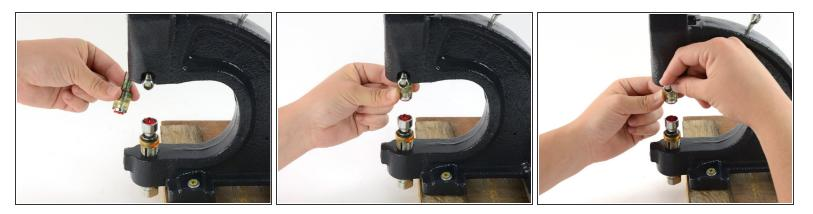
Insert the stud fitting into the upper fitting holder of the hand press.
