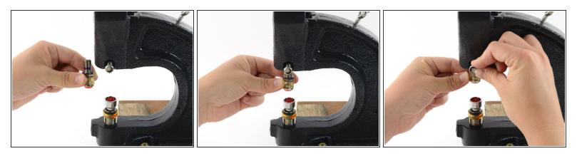
• Insert the socket fitting into the upper fitting holder on the hand press.
