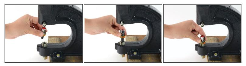
• Insert the cap fitting onto the fitting base of the hand press.
