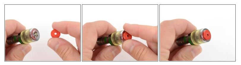
Insert the stud into the stud fitting for the hand press. The widest part of the stud should be facing out. When seated correctly, the stud should snap into place and sit in the fitting without being held.
