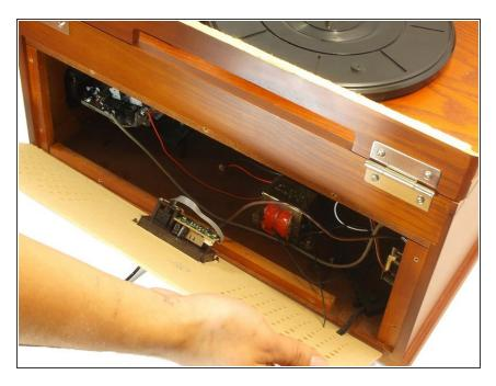
Gently remove the back panel of the device being careful not to unplug any internal wires.
