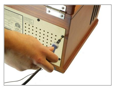
Using your Philips head screwdriver, remove the 10 outer black screws from the back of the device.
