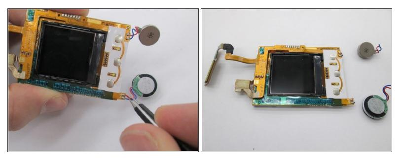
Use a pair of tweezers to disconnect the speaker wires from the circuit board. Note that the soldered connection must be broken for this to occur.
