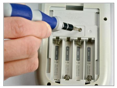
Using the Phillips #00 Screwdriver, unscrew the 15 mm screw holding the backup battery cover, located above the main battery area.
