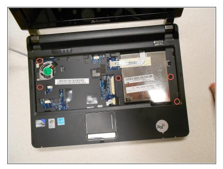
Remove the five (5) 5mm screws shown here using the Phillips #0 screwdriver.
