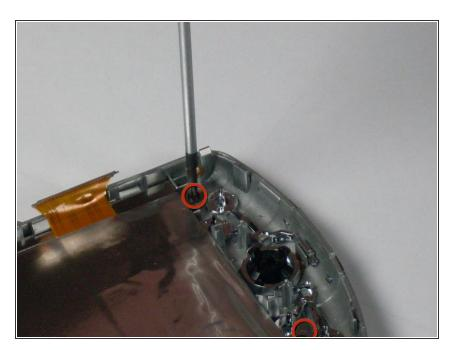
Unscrew the two bottom screws on LCD screen that were previously located under the main board.
