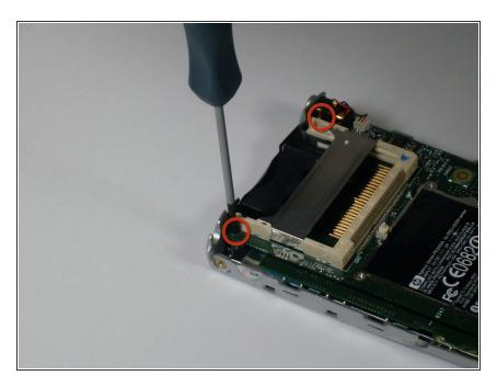
• Unscrew the 2 screws located at each top corner of the main board.
