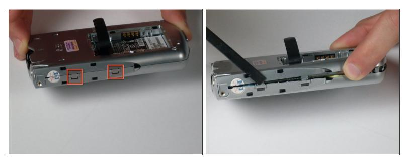
• Remove the back faceplate by pushing and loosening the 4 side slots (2 on each side).
