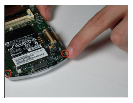
Remove the main board by pushing outward on the two tabs located on each side near the bottom of the device.
