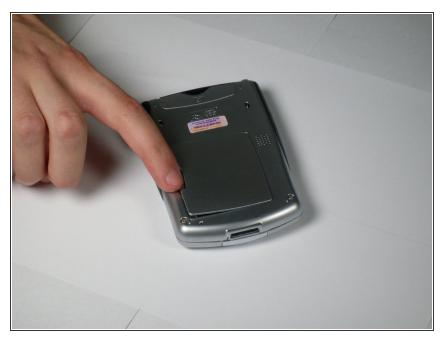
• Press and slide the battery cover tab to remove battery cover.
