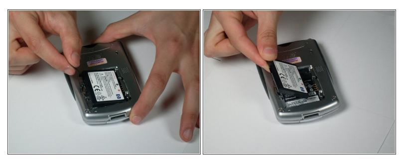
• Pull on the black tab to lift the battery out of the battery compartment.
