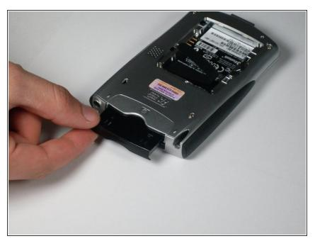
• Remove the CF card by sliding it out of the slot at the top of the device.
