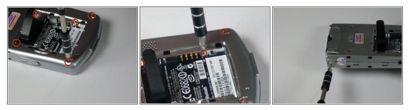
Using the T5 Torx screwdriver, remove all six screws on the back and all screws on each side of the device.
