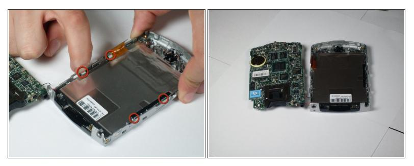
• Press on side tabs to loosen and remove the LCD screen.
