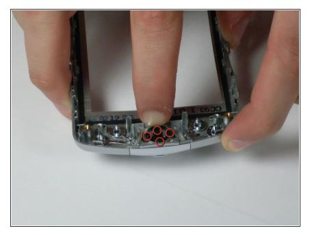
Press on the four joypad tabs on the back, and push it through and out the front.
