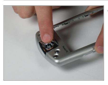
Push the new joypad through the hole; the tabs will lock it into place.
