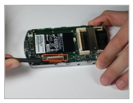
Open the LCD connector, where the orange strip attaches to the main board.
