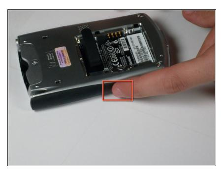
Press down and push the black side strips toward the top of the device to remove them.
