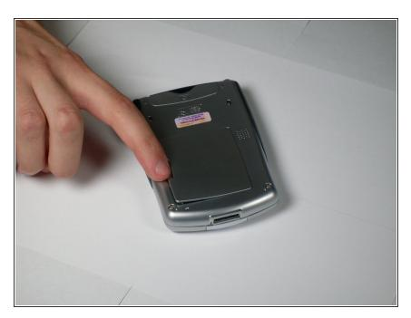
Press and slide the battery cover tab to remove battery cover.
