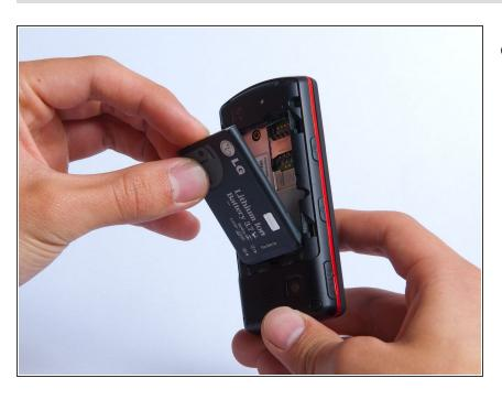
Lift and remove the battery.
