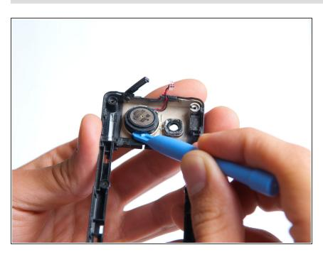
Use the plastic opening tool to pry the speaker out of the back cover.
