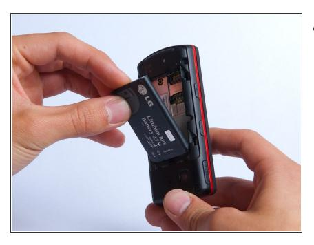
Lift and remove the battery.
