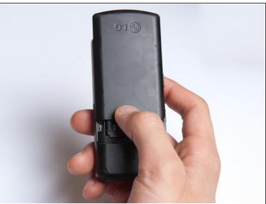
On the back of the phone, place your thumb on the three raised bumps and slide the back cover upward.
