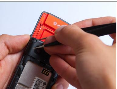
Remove the two screw covers at the top of phone with tweezers.
