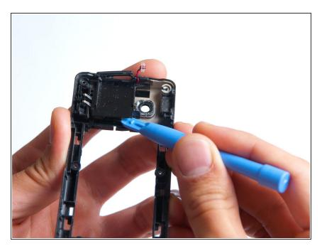
Use the plastic opening tool to pry the speaker cover off of the phone.
