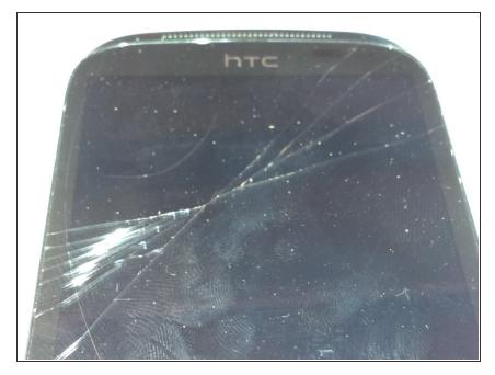
Here is the Desire X, with the touchscreen damaged, but working. I have tried to replace only the touch, but I broke the LCD... It's very very hard to separate...
