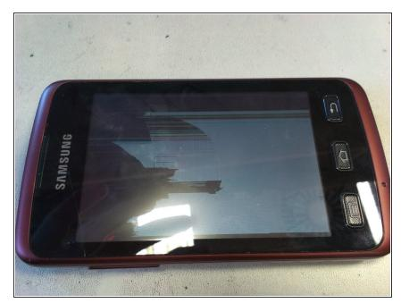
Here is the Samsung Galaxy Xcover, with the LCD broken, that will be replaced.
