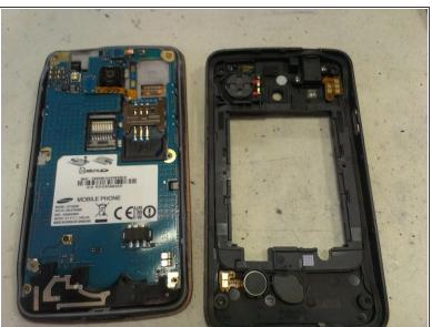
With a flat screwdriver or plastic opener, separate the front case from the rear case. It will be easy!
