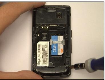
Use a small Phillips head screwdriver to remove the six 3mm screws identified in the photo.
