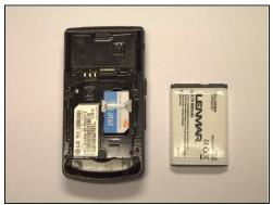
Holding the phone in one hand and using your index finger on your other hand, remove the battery from the phone by prying it out at indention located at the bottom of the phone.
