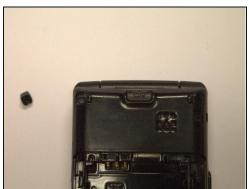
Using a spudger or other sharp tool, remove the two rubber pieces on the top of the back of the phone.
