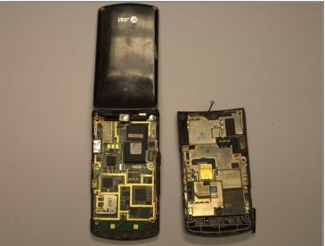
• Use <u>tweezers</u> to carefully unplug the wires connecting the speakers to the mother board.
