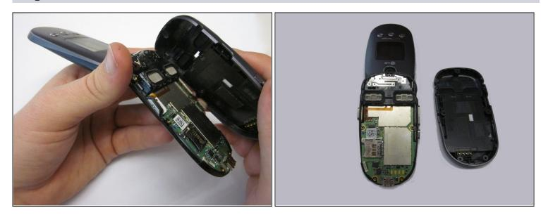
• Remove the back cover completely from the phone.
