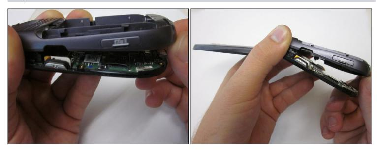
• Lift the back cover starting at the bottom of the phone.
