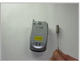
Unscrew antenna from the phone using and clockwise twisting motion.
