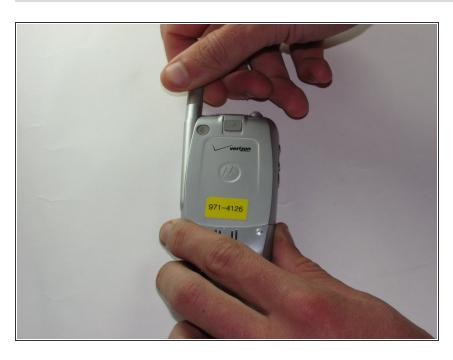
Secure the new antenna onto the phone by re-screwing it on.
