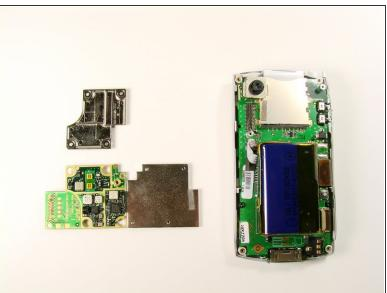
• Use the spudger to lift the logic board from its socket. Remove it from the rest of the phone.
