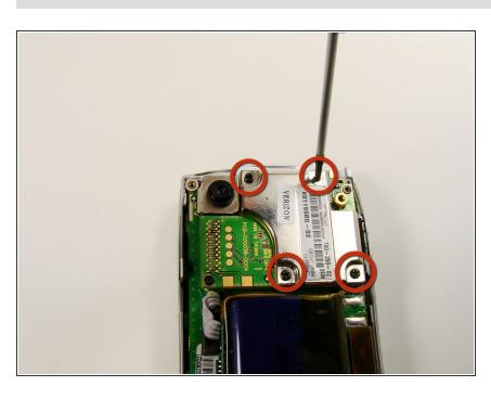
Using the Phillips #00 screwdriver, unscrew the 4 screws holding the silver casing down.
