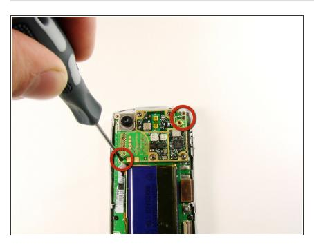
With the silver casing removed, unscrew two black screws with a #00 Phillips Screwdriver.
