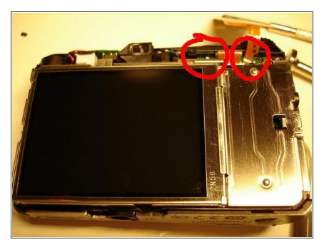
First you need to remove the back cover of the camera, so that you can access the motherboard. Here is how it looks like with the backcover removed (4 scew removed for a powershot A1200). At the top, you can see the main pins connecting the battery contact to the motheboard, but it is difficult to access them.
