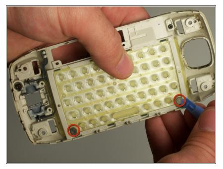
Remove both black "rivets" from the back of the case with the plastic opening tool.
