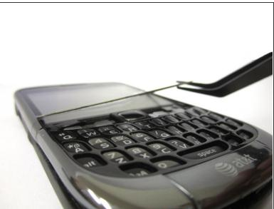
Place the phone face up and use tweezers to securely grip and lift the screen upwards.
