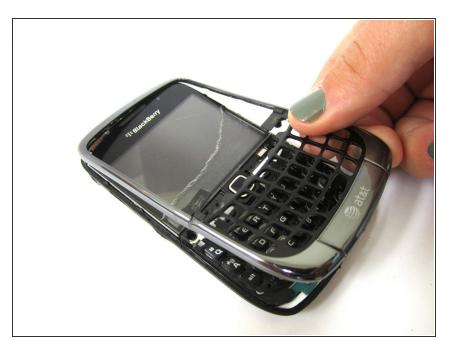
Lift and remove the frame.
