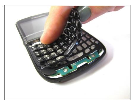
Lift and remove the keyboard.
