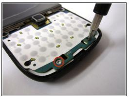
Locate and remove the four 5mm screws on the top and bottom of the phone with a T6 Torx screwdriver
