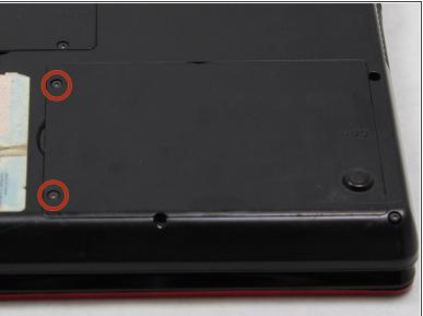
Unscrew the two 3.65mm Phillips #1 screws on the plate marked "HDD".
