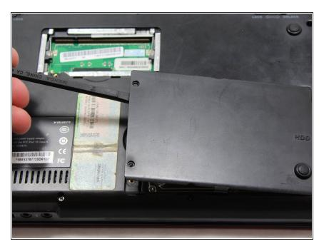
Lift the HDD plate off of the back to reveal the hard drive.
