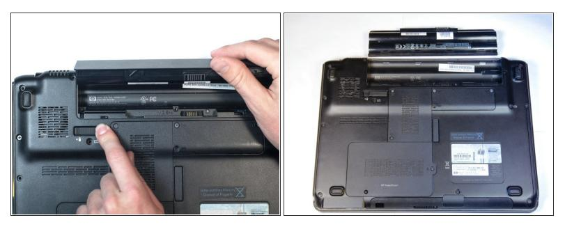
• Step 2: Using the edge of the battery that has popped up, lift the battery out of the computer.
