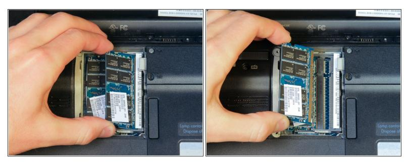
• Using one hand, pull the RAM up and to the left to remove it.
