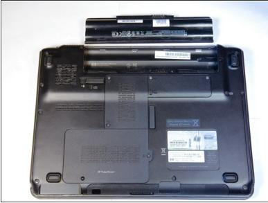
Step 2: Using the edge of the battery that has popped up, lift the battery out of the computer.
