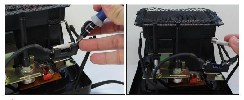
$\triangle$  Do not pry from the middle of the fuse because some fuses are made of glass.
