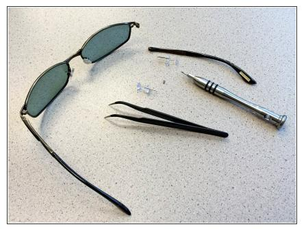
These are the tools I used to insert the screw through the spring hinge. In the video a paperclip was used, but the paperclip I had on-hand could not fit into the tiny recess in order to jam the spring open.
