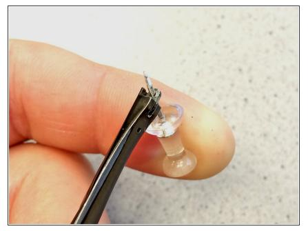
Insert a pushpin through the hole and use it as leverage to extend the spring hinge outwards.
