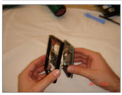
Now that both ribbons and the wire are disconeccted, you can apply a downward pressure to the battery. You will have to carefully rotate the frame so that the battery can go through.
