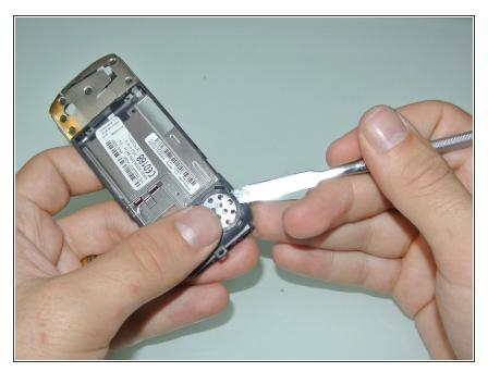
Insert your metal spudger to remove the metal plate and free the upper speaker.
