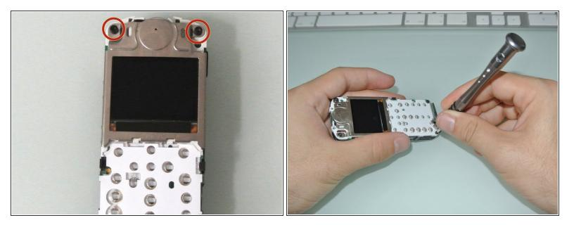
Remove the 4 T6 Torx screws
