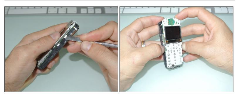
Use a metal spudger to pell off the four metal clips and separate the motherboard and keyboard from the main plastic part.
