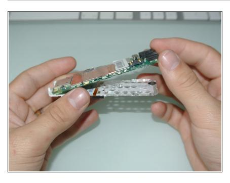
The last thing you need to doto access the Logic Board is to separate the Keyboard/Screen block just taking apart with your fingers. To reassemble your device, follow these instructions in reverse order.
