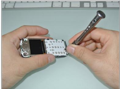
Remove the 4 T6 Torx screws
