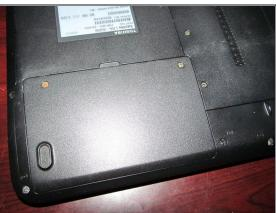
• Screw the hard drive cover on the laptop. Once it is screwed in, snap it down to secure it.
