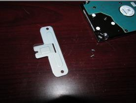
• Remove the hard drive mounting bracket. Loosen the 2 highlighted screws to remove it from the bracket.
