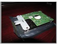
Screw the hard drive bracket on the new hard drive.
