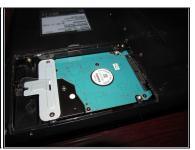
• Remove the screw holding the hard drive in the computer. Slide the drive backwards to remove it from the laptop.
