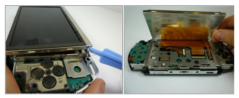
• The LCD Screen is held by the LCD Frame with similar clips. Slide a thin tool between the clip and the screen and gently pry them apart while beginning to lift the screen.
