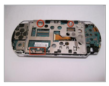
Remove the screws on the top and bottom of the frame. Be sure to keep track of where you took each screw out of.
