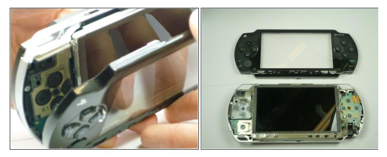
• Gently separate the outer plastic casing from the rest of the system as shown.
