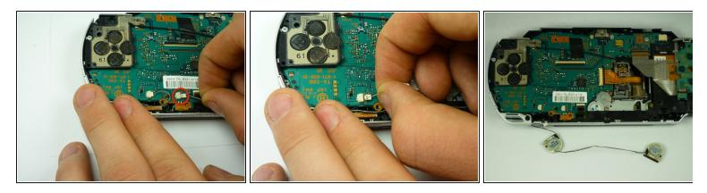
• Gently unplug the speakers from the socket. The speakers are completely detatched when they are unplugged from the logic board.
