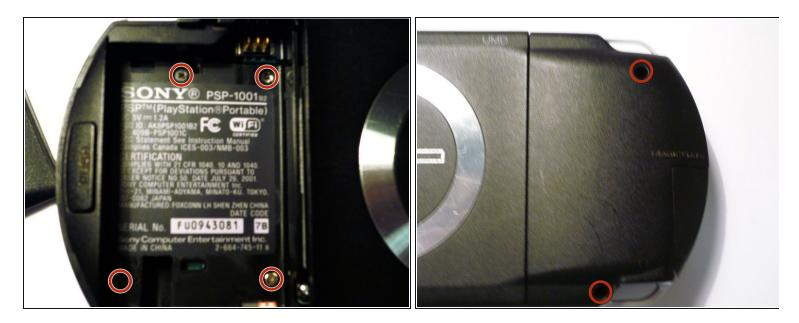
• Remove the four screws shown with a Phillips #00 screwdriver.
