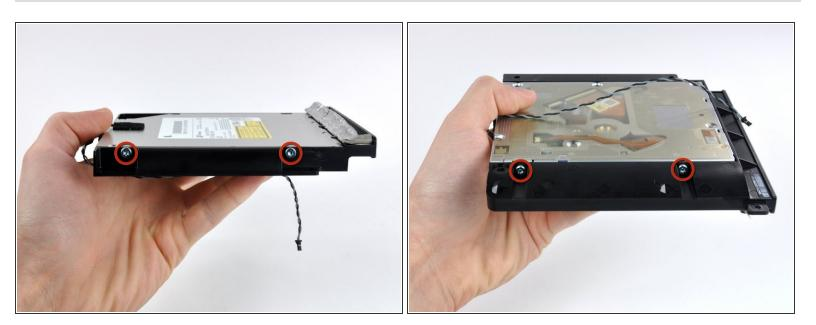
• Remove the two T10 Torx screws from both sides of the optical drive (four screws total).
