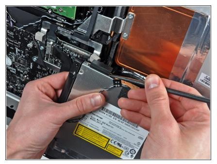
• Use the flat end of a spudger to help disconnect the optical drive cable.
