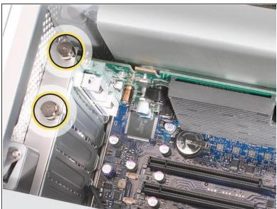
This procedure explains how to remove a standard card and a card that includes a booster cable. Before you can remove either type of card, however, you must first loosen the two captive screws that secure the PCI bracket to the enclosure and remove the bracket.
