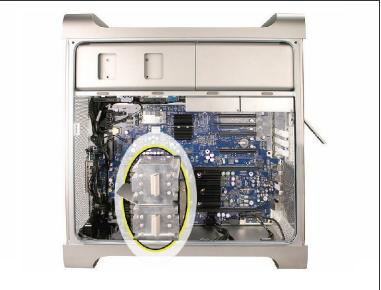
Disconnect the 2-pin cable for the upper processor (CPU A) heatsink from the logic board.
