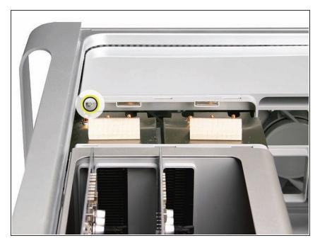
Remove the second Phillips screw at the bottom front of the assembly.
