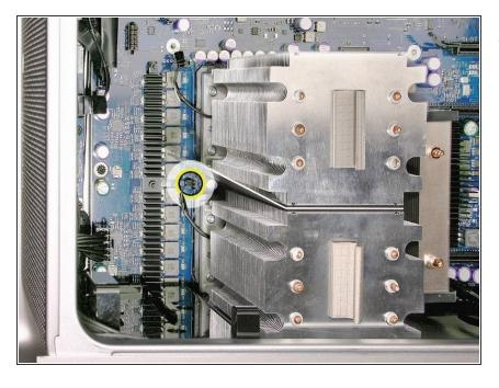
Disconnect the cable connector for the lower processor (CPU B) heatsink.
