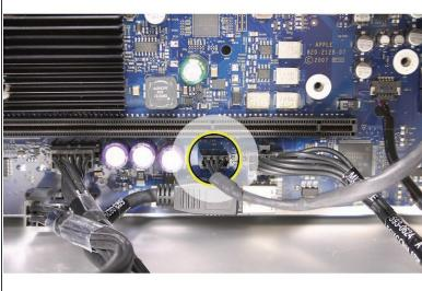
Disconnect the rear fan cable from the logic board.
