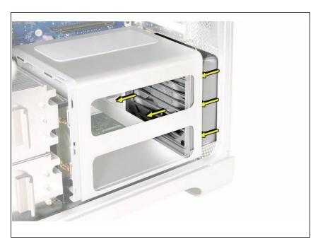
Slide the rear fan into the memory cage.
