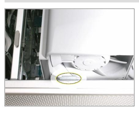
Replacement Note: Also make sure the latch on the inside top left edge of the fan assembly engages with the slot on the inside lip of the enclosure
