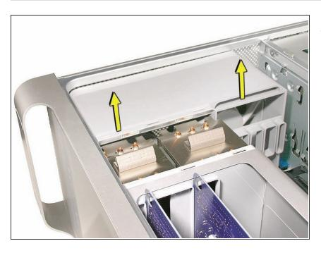
Place one hand on each end of the fan, lift straight up, and remove the fan from the enclosure.
