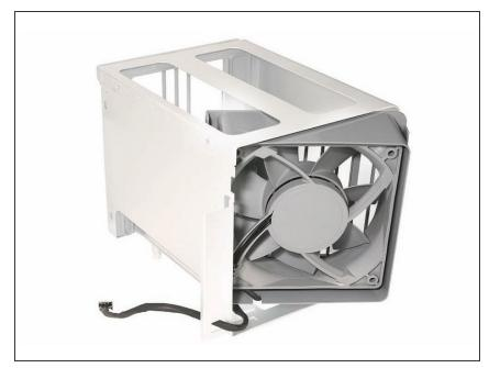
(i) Replacement Note: If you are installing a new fan in the memory cage assembly, rotate the fan into the cage as illustrated. Also note carefully the orientation of the fan in relation to the cage.
